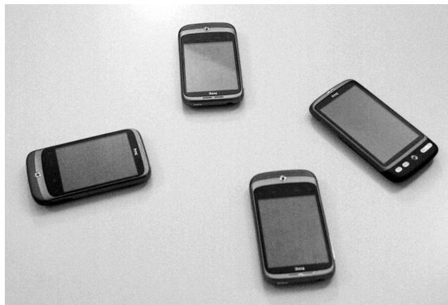
**Fig. 1:** An exemplary ad hoc array comprised of four commercial off-the-shelf smartphones.
